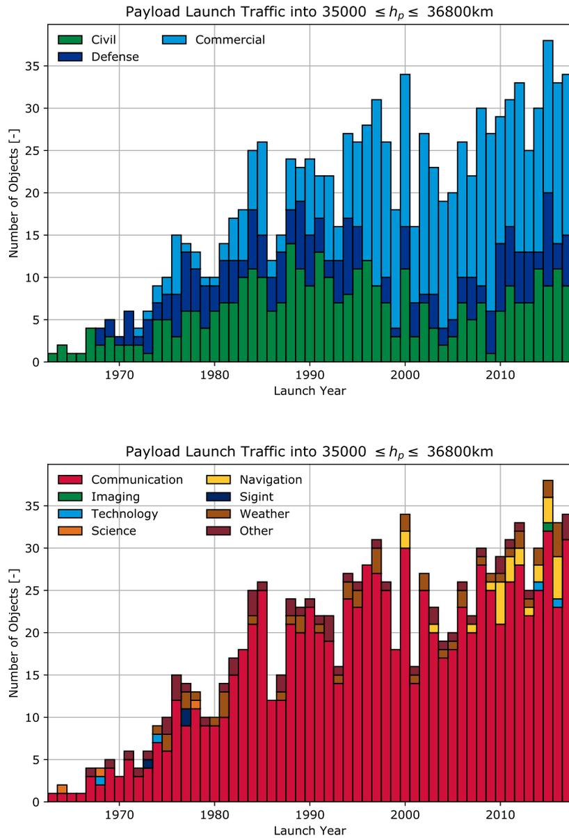
Figure 2.8: Evolution of the launch traffic near  $GEO_{IADC}$  per mission funding (top) and type (bottom).
