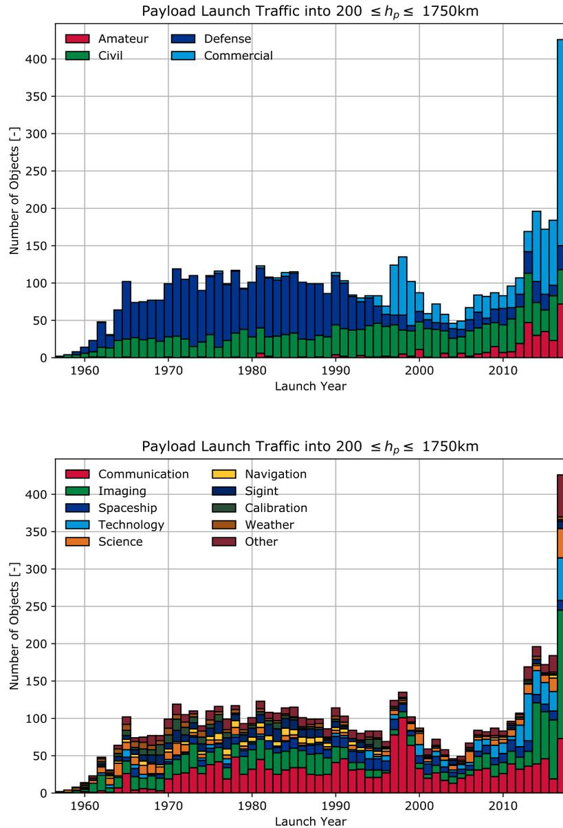
Figure 2.7: Evolution of the launch traffic near  $LEO_{IADC}$  per mission funding (top) and type (bottom).
